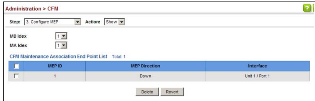
Figure 346: Showing Maintenance End Points
