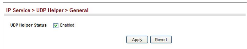
Figure 495: Enabling the UDP Helper
