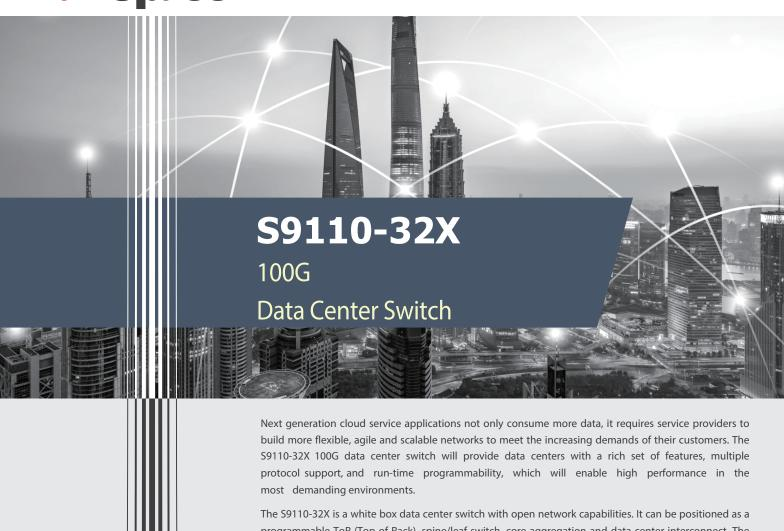
The S9110-32X is a white box data center switch with open network capabilities. It can be positioned as a programmable ToR (Top-of-Rack), spine/leaf switch, core aggregation and data center interconnect. The load balancing and congestion management from the S9110-32X enables it to be positioned as an application load balancer.
