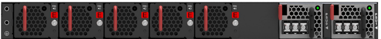
(Front-to-Back Airflow Fans)
